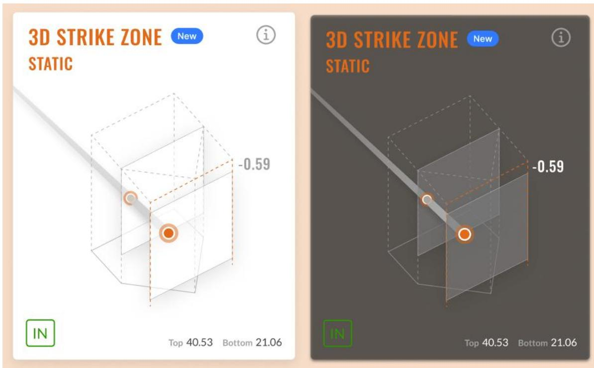
If a pitch is considered “In” then the user will see an orange ball marker where the ball crosses each plane that is in use. If the ball misses the entire area of any of the planes it will be considered “Out”, and the user will see a gray ball marker on any plane that the ball misses.
